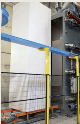
Block moulder with new waterless vacuum system
