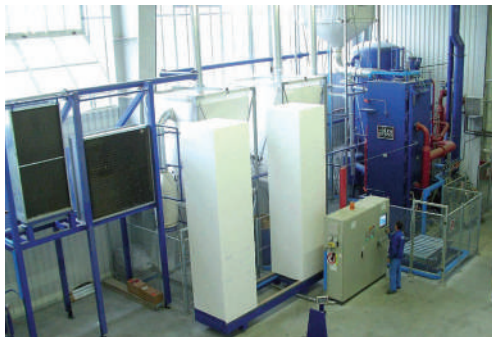
Benefits of a vertical mould are density uniformity and a low degree of residual humidity present in the blocks
