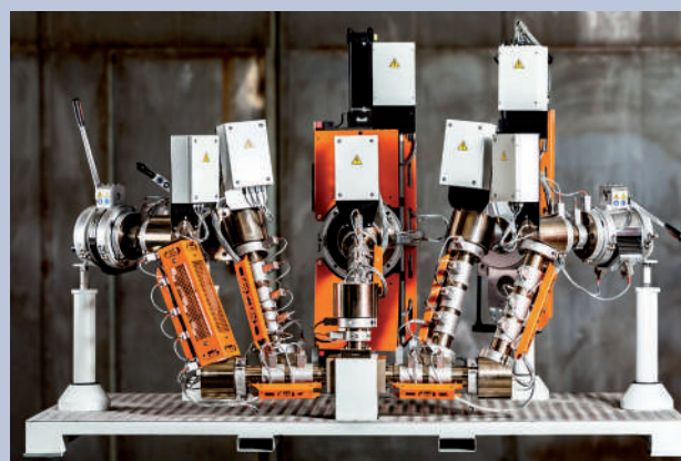
For a 5-layer cast extrusion line BD Plast has developed a group of fittings and elbows preinstalled on a dedicated platform and each equipped with a different single-plate screenchanger
