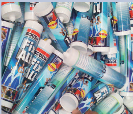
The DHDT system from GMC permits to directly print chemical and food packaging, flexible tubes and sealant cartridges starting from a file
