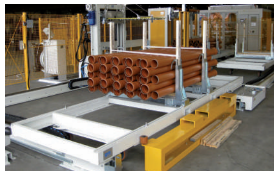
An IPM plant for packaging and palletizing pipes
