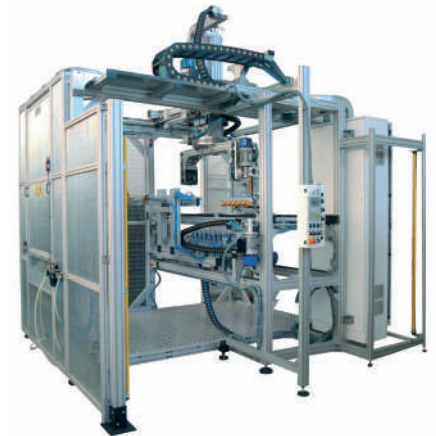
The cell developed for the production of rubber bellows
