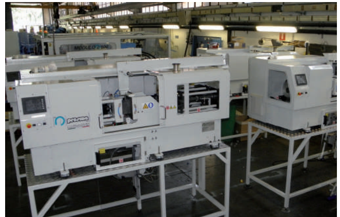
The new Presmall SC 6 distinguishes itself from the previous model mainly for the 6-ton tiebarless clamping unit and the multi-axis control system driving up to 16 axes
