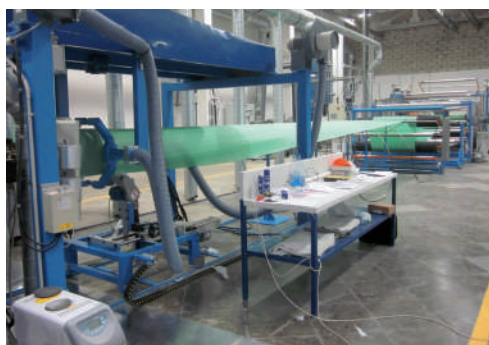
FAP can now design and build machines which output ranges from 50 up to 1,500 kg/h, obtaining very low density, such as under 16 kg/m 3
