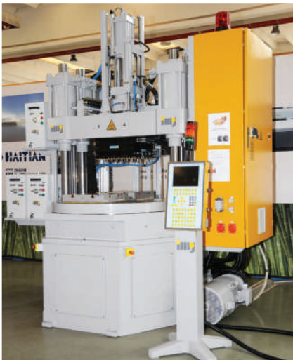
150-ton vertical press featuring rotary table with two temperature-controlled platens for the overmoulding of inserts
