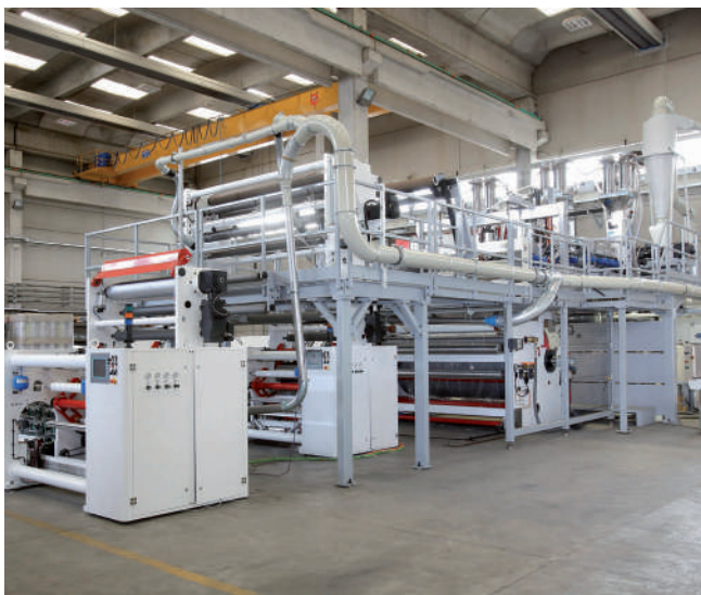
The new stretch film winder for the production of either hand rolls, or machine rolls and jumbo rolls, shown by Dolci Extrusion at the K Show
