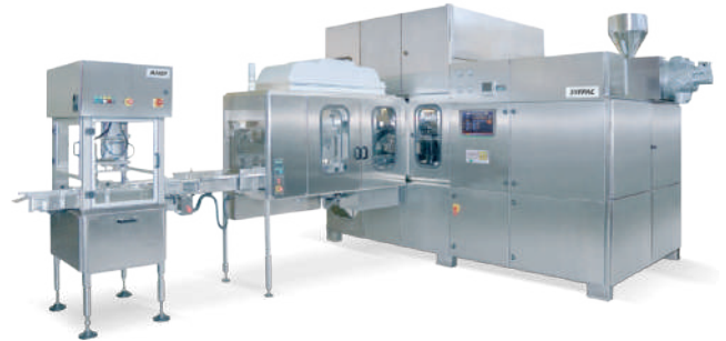
The Secureject machine allows the production of prefilled syringes in 18 seconds at a cost of 12 euro cents starting from the polymer
