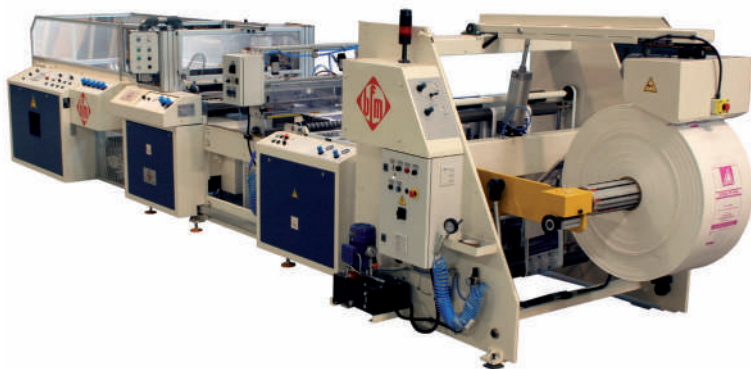
The BF-106 HS 800 automatic bagmaking machine is equipped with a motorized unwinder unit for reels with a diameter up to 1,500 mm
