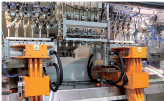
The extrusion head of the PB10E/DXL blow moulding machine has been designed to allow a greater control of the extruded parison and permits color changes in less than half an hour
