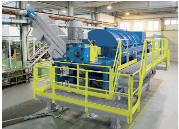
The new unit for removing shrink labels from post-consumer PET bottles in washing and recycling plants
