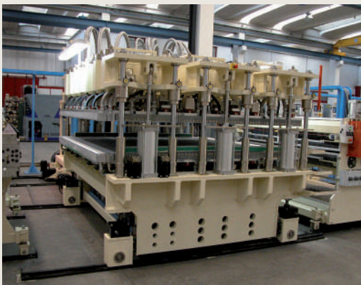
The calibration unit developed by BG Plast Impianti is intended for processing both PC and PP hollow corrugated sheets
