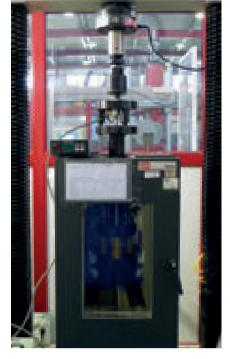
Within TDM-Seals project, a particular test rig has been developed to measure demoulding forces in a rubber cubic sample. The test rig is implemented in a Universal Testing Machine (UTM) with a climatic chamber, in order to assess the influence of different mould surfaces or coatings on the demoulding process
