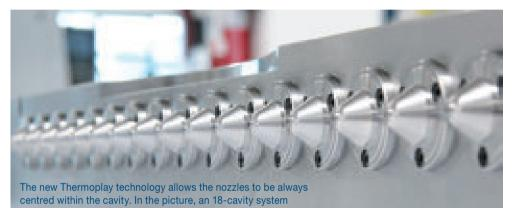
moplay nozzles are provided with plastic sealing zones in order to avoid any plastics leakage and to guarantee a high-quality injection point on the preform.
