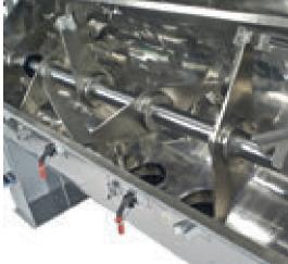
The inside of the CMX high efficiency horizontal cooler
