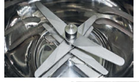
The innovative design of the mixer tool permits greater friction and mixing intensity, while new antiwear coating guarantees longer life
