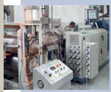
The new line developed by Bausano for the extrusion of plastic wavy profiles for roofs (PVC tile sheet)
