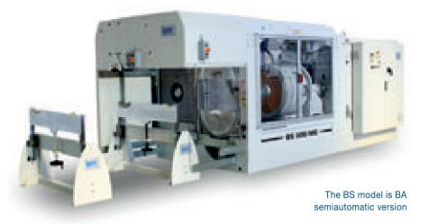
the pipe being heated is constantly kept under control by sensors allowing the monitoring and control of the entire heating process, so that the heater is turned off when the desired temperature is reached, which means significant savings. To guarantee uniform heating in all the points, the pipe rotates around its own axis by means of specific rollers.
