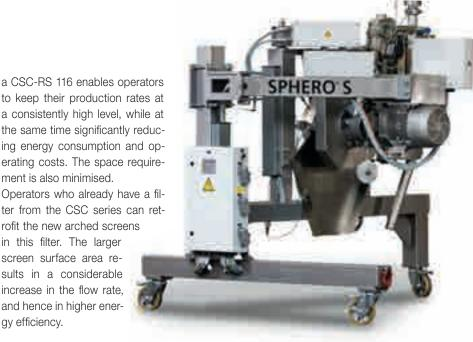
The newly developed Sphero S underwater pelletizer is the heart of the system developed for polymer production in the mid-tier throughput range
