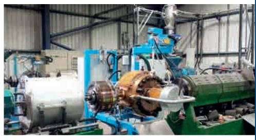
Plasgran has three 400 Fimic filters installed on all of the pelletizing lines. The most recent addition consists in a filter equipped to work in both scraping and backflushing modes, for very fine filtration
