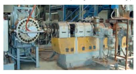
Idealservice is able to produce 20,000 tons of granules and 15,000 tons of SRA (Secondary Reduce Agent), with a recycling rate of almost 90%. It has been able to reach this results also thanks to two Fimic self cleaning filters with a diameter of 500 mm
