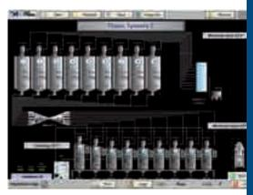
Screen for the supervision system, material storage, drying and centralised feeding
