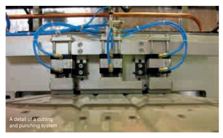
erance of up to 0.2 mm on the length and ensures lower energy consumptions. The unit can be equipped with different tools, according to the pipe material, and can reach speeds up to 25% higher than traditional cutting machines.
