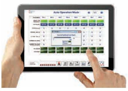
The HRSflow FLEXflow controller grants accurate setting, control and monitoring of the valve pin position, speed, acceleration and stroke.
