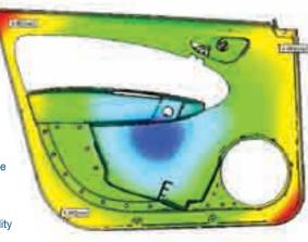
cess, pressure in the part is more even and peaks are reduced, and the part thickness is more uniform. This brings a weight reduction. The holding pressure can be adjusted independently for each nozzle, obtaining more uniform pressure distribution. This minimizes the bending of the mould. Reducing the stress in the mould, also the required stiffness is reduced, allowing steel saving in the tool production.
