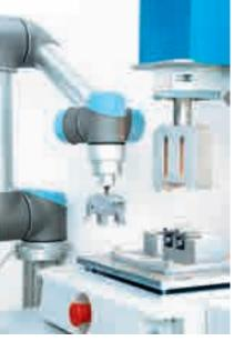
VDMA Blue Competence concept study for Fakuma 2014: standard modular ultrasonic welder HiQ Dialog with small-scale robot: handling, testing, welding, and marking of a toy elephant
