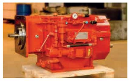
Zambello is specialized in the design and manufacture of gearboxes for extruders and injection moulding machines
