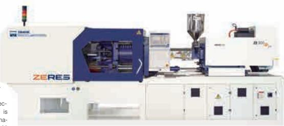
For the launch, the Zeres range is available with clamping forces of between 40 and 230 t
